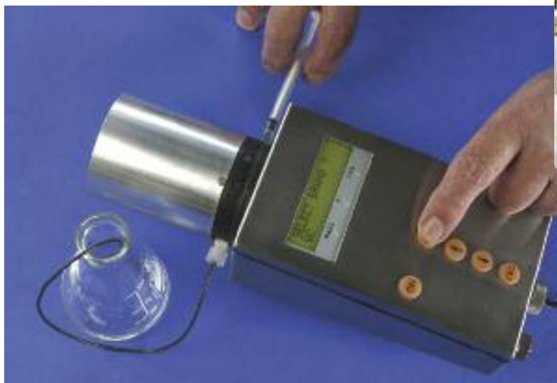
The SAD Brand Authenticator®, a small-hand held UV/visible spectrophotometer designed for investigators to use in the field.
